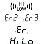
'Hi' or 'Lo' is displayed when the temperature being measured is outside of the settings of HAL and  ${\sf IAI}$
