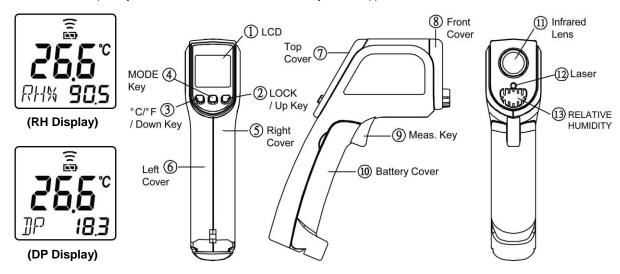
Simply aim the thermometer at the measure target with Lens  $(\bigcirc, 11)$  and press Meas. key  $(\bigcirc, 9)$  to display the surface temperature. The Distance:Spot is 12:1. Please make sure the target area is within the field of view.
