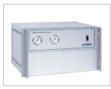
The Michell PSD Series Pressure Swing Dryers use two columns filled with 4Å molecular sieve desiccant, which are used alternately on a two-minute switching cycle. The PSD dryers are designed to operate continuously, using a small proportion of the dried air, to regenerate the offline column - generally giving desiccant life in excess of five years. This type of heatless regeneration also uses significantly less energy than a 'heated' type of dryer.
