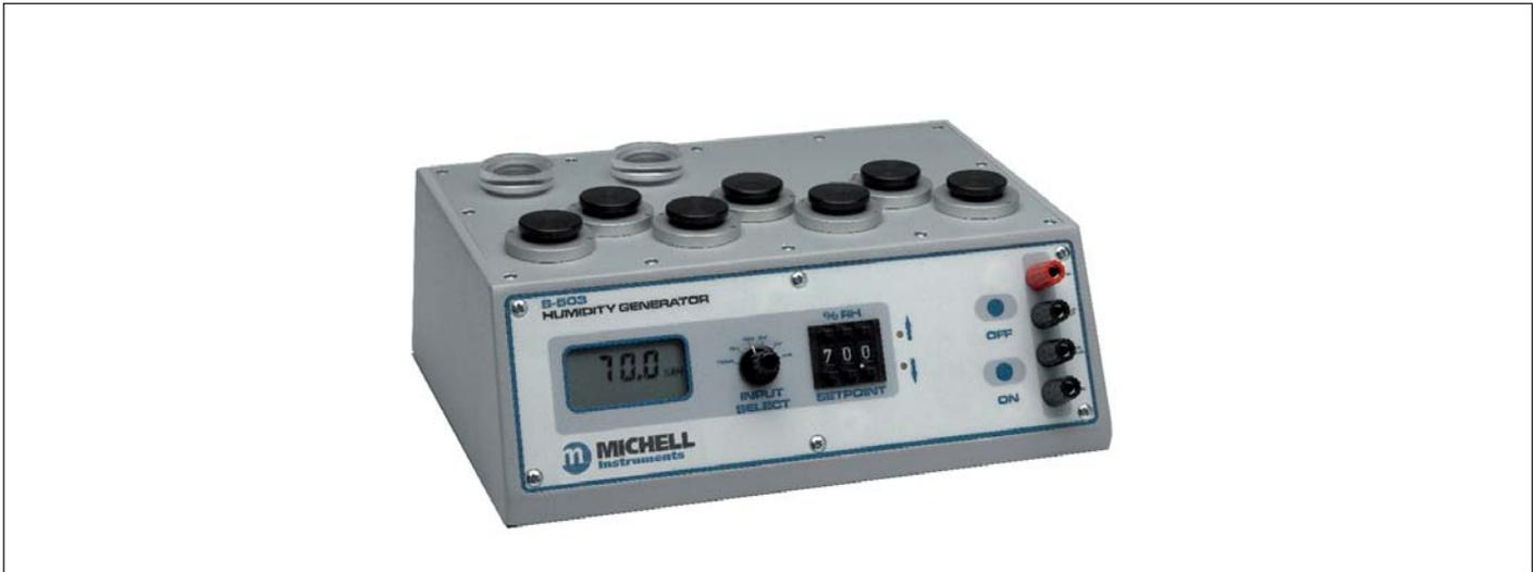
The S503 is a highly portable and compact self-contained bench-top humidity calibrator. The humidity controlled chamber features interchangeable ports accommodating up to 7 humidity sensors and is ideal for companies or organizations that need to calibrate large numbers of probes in the field.
