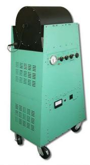
The LS3000 Series Blackbody Source has a 0.5" or 1.0" diameter cavity and is continuously adjustable from 1000°C to 3000°C. A dry argon gas atmosphere is required.
