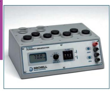
The S503 Humidity Calibrator enables users of humidity sensors, transmitters and portable devices to quickly and accurately generate a stable humidity in a test chamber to validate or calibrate sensors.
