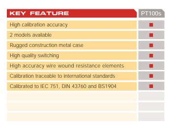
Designed for the accurate and reliable simulation of platinum resistance thermometers (Pt100), the simulators Pt100S/2 and Pt100S/1 offer 2 low cost options. Both models are calibrated to international standards.
