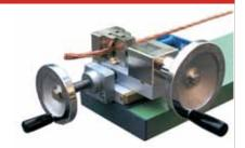
Measurement length: 1000mm. Clamping device: designed for cross sections of 1mm² to 1000mm². Distance between voltage and current-clamp: 420mm. Dimensions (height x width x depth): 170mm x 2100mm x 250 mm. Weight: Approximately 25kg.
