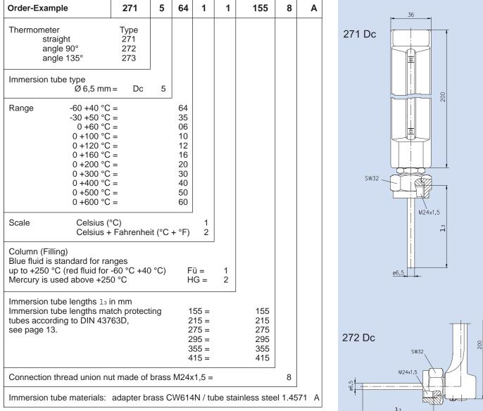
On principle, thermometers of type Dc are supplied with a steel immersion tube of  $\emptyset$  6,5 mm for the lower part of the capillary, which fits into protecting tubes with 7 mm bore.
