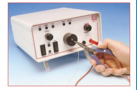
The L60+ is designed for sensor manufacturers for the production of commercial grade thermocouple junctions, and for users of large numbers of exposed junction thermocouples such as test and development laboratories where multipoint temperature sensing of test pieces is required.
